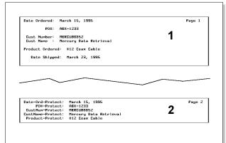
**Figure 1.** Sample Q&A for DOS data entry form with two pages. Only the Date Shipped field on page 1 is editable during update. The fields on page 2 are read-only and inaccessible.
